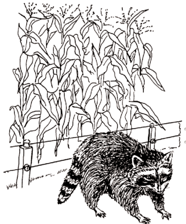
Figure 1. A simple two-wire electric fence
